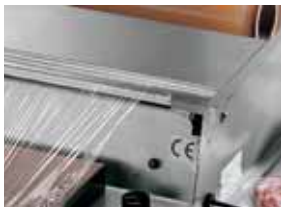
Particolare filo caldo (1) Heated cutting tread (1)
